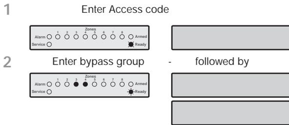
3 The keypad will display the bypassed zones. If required, zones can be added or removed from the group by entering the required zone number, e.g. Enter to add Zone 5.
