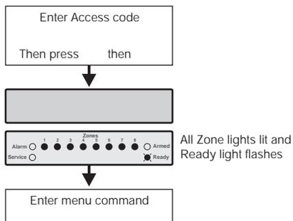
A programming menu is selected by entering a two-digit menu code. On completion of each menu option, the system reverts to the main programming menu, allowing other programming menu options to be accessed.
