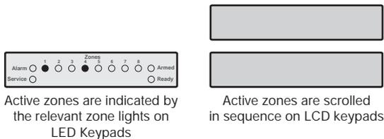
!! If any unbypassed zones that are not enabled for "Force Arming" are violated at the end of the exit delay this is termed an exit error and the alarm system will go into fail set state (internal alarm). If programmed by the installer the external bell will also sound. Enter a valid user Access code to silence this alarm.
